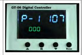
When the temperature shows on the display is not the same as actual temperature on heat platen, press on button for 5 seconds to reset mode:
