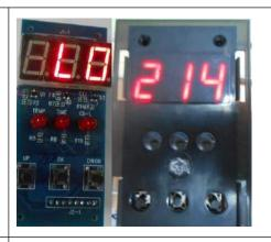
When rising to the set temperature, close down the heat platen and time controller starts to countdown.. Tips: it will show LO when temperature is below 100°C.
