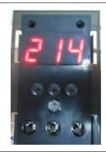
Once the time is up, the buzzer will send out sound. Then open the heat platen
