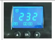
When it close the mug heater and start to transfer, the time starts to count down, once time is up, mug heater open automaticlly and start the next cycle.
