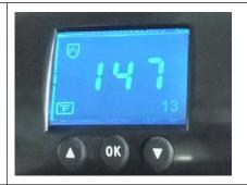
Press button after time setting; the display shows the temperature starts to rise. When the temperature rises to the setting temperature, the buzzer sends out sounds; then put in the mug and starts to transfer.
