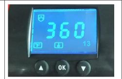
Press button, the temp light is on. Select with arrows the temperature according to different transfer material (such as 360°F).
