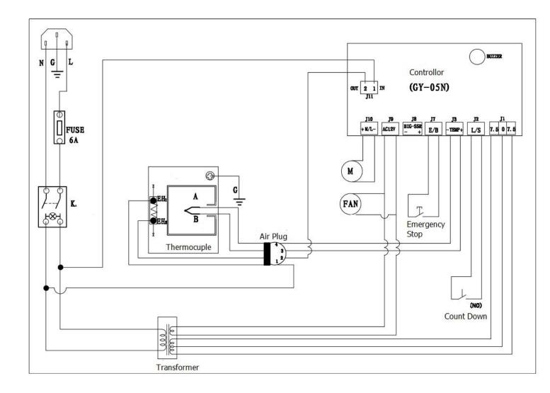
K<sub>0</sub>: Power Switch SJ: Digital Controller FU:Fuse R1:Relay T: Transformer
