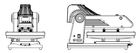
Model No. : E-15S/E-20S Description: Electric powered fully auto heat press Heat platen sizes: 380x380mm (15"x15") / 400x500mm (16"x20") Voltage: 110V/220V single-phase Power: 1.6KW/1.8KW Temperature range: 0-255 °C (0-490 °F) Time range: 0-999S Pressure range: 0-10 Printable articles thickness: 0--20mm
