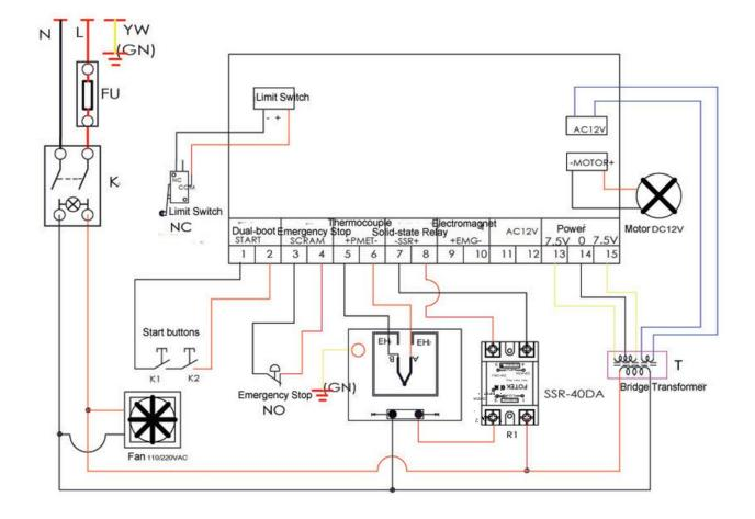
K.: Power Switch T: Bridge Transformer EH1 EH2: Heating Pipe K1 K2: Start Buttons
