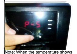
on the display is not the same as actual temperature on heat platen, press button for 5 seconds to enter the P5 mode:
